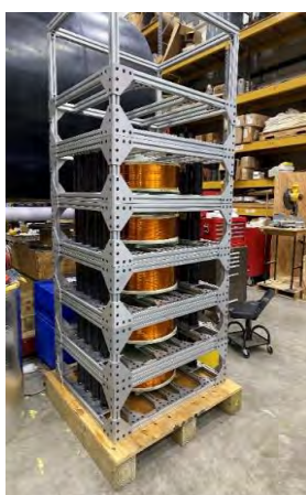
Figure 4.6.2.1.4: The PFN fabricated in-house and the output waveform during TC1 testing.
