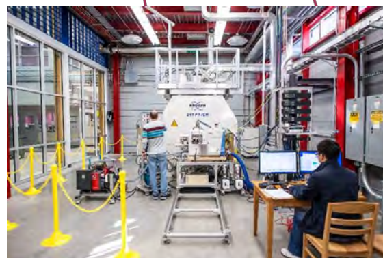
Figure 2.2.5.2.1: Picture of the 21T FT-ICR mass spectrometer.
