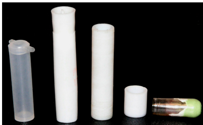
Fig. 2. Typical sample containers for non-air sensitive powder or solution samples in the homodyne transmission spectrometers. From left to right: Fisher brand vial 03-338-1A; a homebuilt teflon container integrated with the support placing the sample at the right height; a teflon support for a sample cup; a 400 \mu L-volume teflon cup; a ‘00’ size gel cap. The outside diameter of all these containers is 8 mm.
