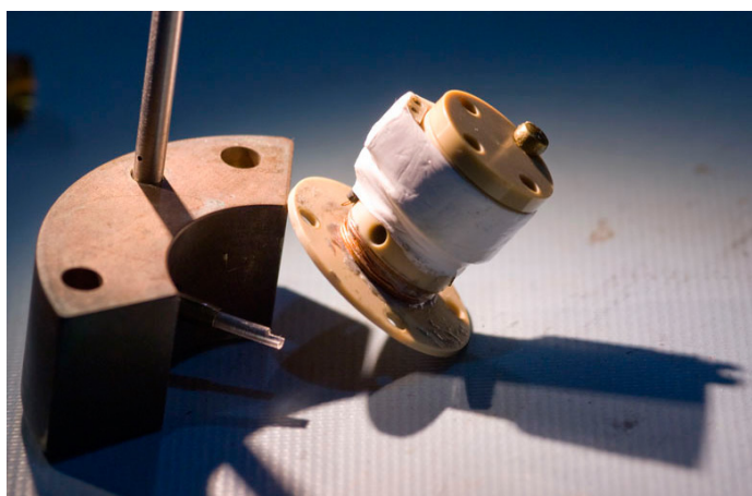
Fig. 5. Single-crystal sample rotator for the heterodyne quasi-optical spectrometer. The 2 mm rod fits sideways into the modulation coil (right).
