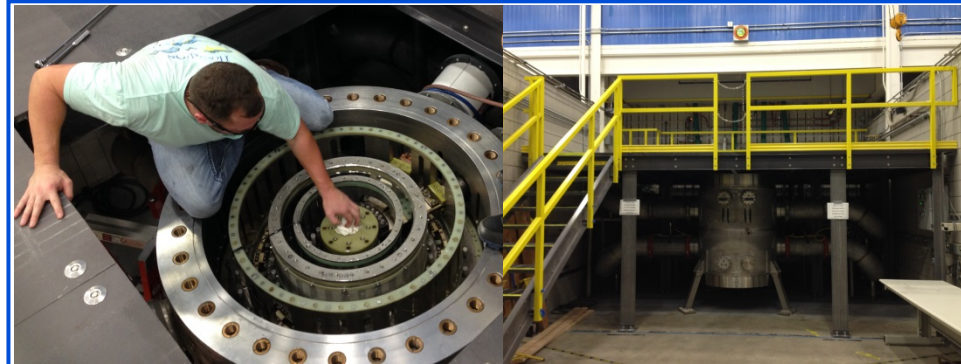
Assembly of the coils and support structure in the one meter housing (above-left).
