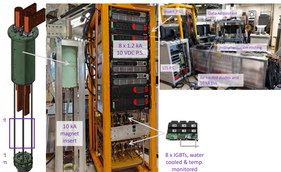
Figure 4.1.18. High current magnet test facility with upgrade to 10kA capability including IGBT solid-state switching for faster active quench protection.
