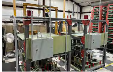
Figure 2.2.7.4. Two modules of the 1.2MJ, 30kV capacitor bank assembled in Alpha Omega Power Technology LLC at the end of 2023.
