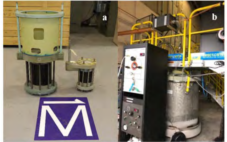
Figure 2.2.7.2: (a) The current 75T duplex magnet made of CuNb (left), next to a standard 65T short pulsed magnet made of AL-60 (right). (b) The cryogenic and experimental platform set-up for the duplex magnet.
