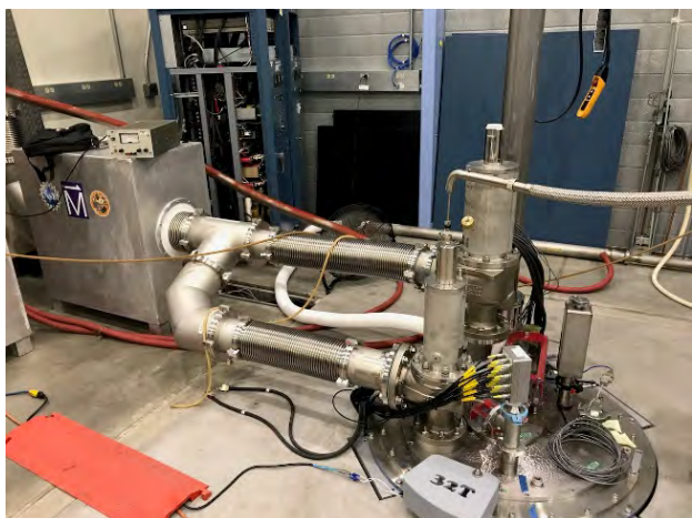
Figure 2.2.2.3: 32T all-superconducting magnet shown during cooldown to 4.2K.
