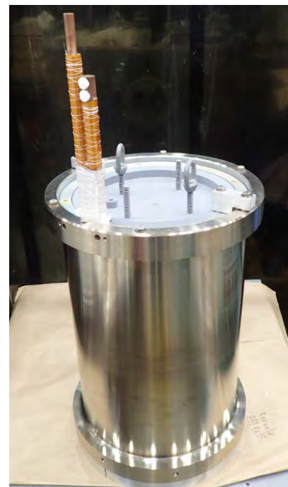
Figure 4.4.18: Coil 2 of the 100T Multi-Shot Magnet with its reinforcing shell, prior to epoxy impregnation.
