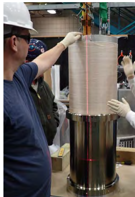
Figure 4.4.17: Coil 2 of the outsert of the 100T Multi-Shot Magnet being inserted into its Nitronic-40 reinforcing shell.
