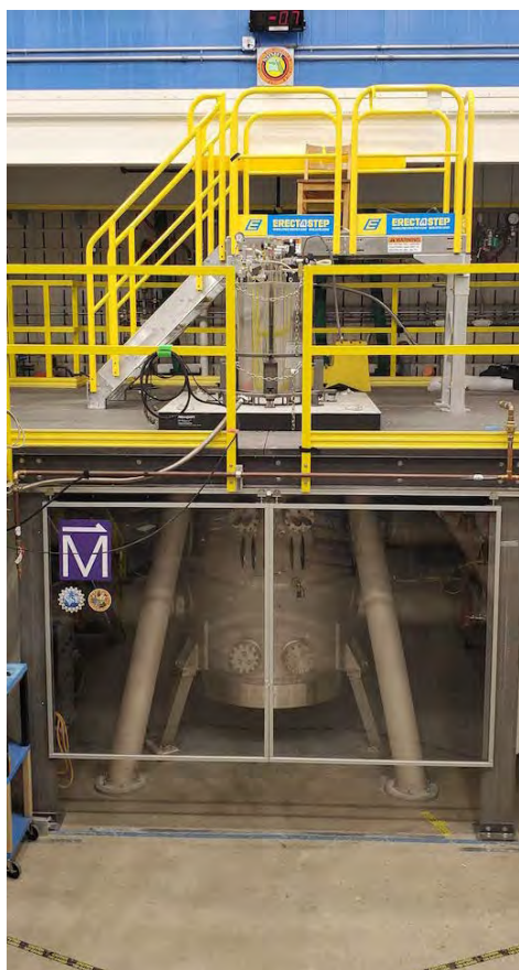
Figure 2.2.2.5: Cell 6 (41.5T) cryostat with advanced vibration isolation.
