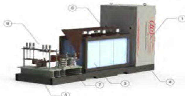
Figure 4.4.15: (Left) Measured waveform of magnet field generated by 75T duplex magnet during the commissioning phase. (Right) the picture of duplex magnet with MOV bank and containment vessel during its testing.
