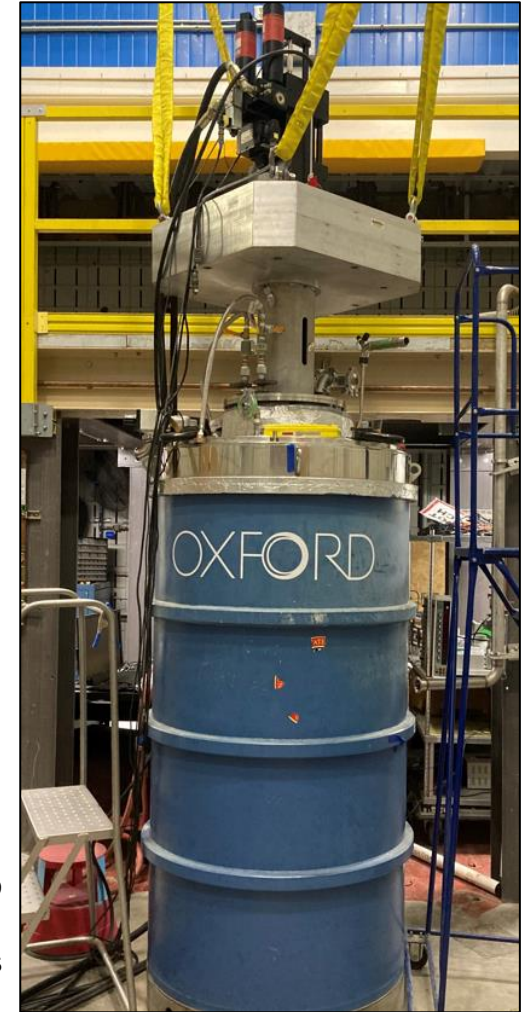
Figure 1 (top): REBCO test coil (red arrow) attached to the load frame that is inserted to test facility at right.
