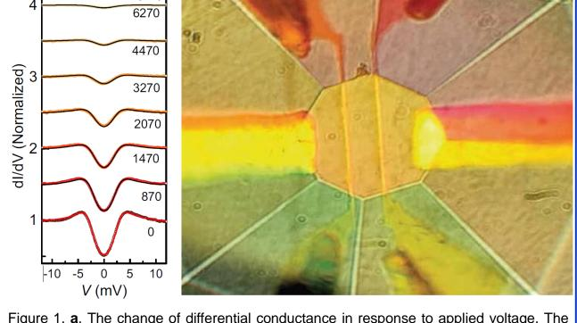
Figure 1. **a**, The change of differential conductance in response to applied voltage. The drop that forms near 0 mV is due to the opening of the superconducting gap. Vertical spectra are offset by increasing magnetic fields values shown on the right. **b**, An image of the tunneling circuit formed on the tip of the diamond anvil press.
