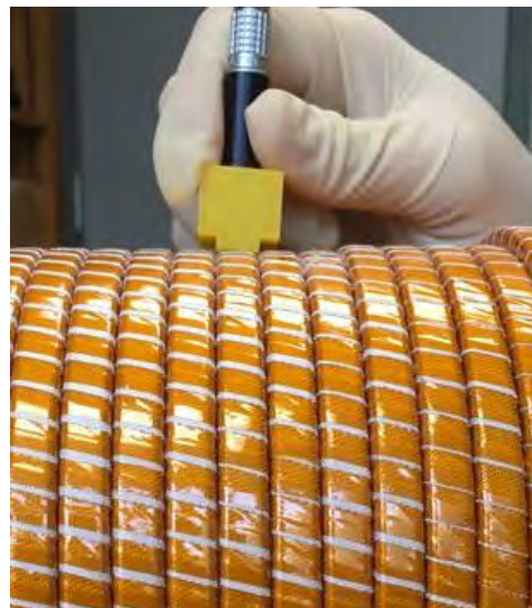
Figure 4.56: The conductor of a large pulsed coil is inspected after winding to verify that no cracking occurred during the winding process.
