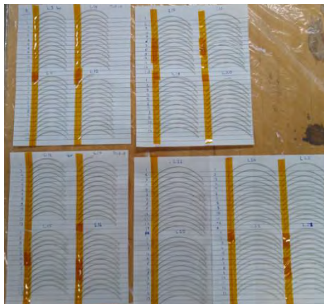
Figure 4.43: Left: Systematically extracted short samples from coil Pup-9 in preparation for short sample transport characterization. Right: A selection of J_e data measured from these samples.
