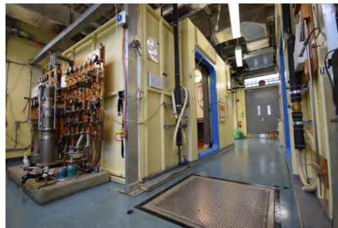
Figure 2.22: July 2021 view of the corridor between the Bay 3 (left) and Bay 2 (right) shielded rooms in the Microkelvin Laboratory. The dilution refrigerator and vacuum plumbing are seen before they pass through an opening to the pumps and containers in the lower floor. As part of the “disinfect/sanitize” protocols, a freshness was restored to the facility.
