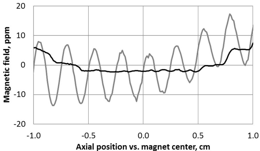
Deviation of field strength along a 1 cm diameter/2.5 mm pitch helical trajectory at 35.2 T, 28.2 T, and 23.5 T (top to bottom): base trajectory (grey) and corrected with combination of passive and active shims (black). Field homogeneity is optimized over the middle +/- 0.5 cm portion and is better than 1.0 ppm over a 1 cm cylinder volume at all three fields.
